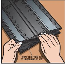
**3.** Remove backing from 1 Peel-&-Stick end cap section. Apply half of the section to end of the vent, starting with the top cap. Wrap other half of end cap down and underneath vent legs and Snow Screen to close off end of vent
