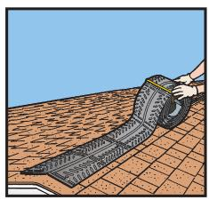
**4.** Beginning at end of ridge, apply vent with minimum 1¾" nails (2 coils provided in box) following "NAIL HERE" guides along vent cap. Only apply nails within the area between leg cavities – DO NOT apply nails outside of "NAIL HERE" guide marks. Vent may be power nailed or hand nailed. Do not overdrive nails. Apply first four nails (two on each side), then remove colored band to unroll rest of vent. Continue to apply according to marked guides. Repeat Step 3 to seal opposite end of vent.
