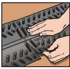
**5.** For runs longer than 20 feet, additional vent rolls can be applied. Line up end of additional vent roll with previous roll by overlapping at offset lip, then apply Peel-&-Stick end cap to seal junction. **Follow Step 4** to apply rest of vent.
